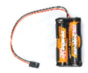
**STEP 2**: Insert the socket of the battery holder wires into the "IN" prongs on the right side of the servo tester. Match up the black wire of the battery holder with the negative (bottom) prong of the servo tester. A blue light at the top of the servo tester should light up.
