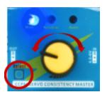
**STEP 5**: *Manual Mode* - Twist the yellow dial on the servo tester back and forth. The servo horn on top of your motor should rotate. The range of motion for servo motors is 180 degrees (half-circle).
