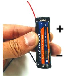
**B)** Attach the AA battery holder on the top of the box using a piece of double-stick foam.
