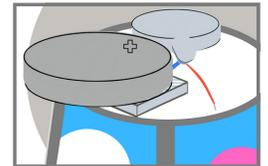
**C 6** Touch the red wire of the motor to the **top of the battery**. You should feel your robot move!
