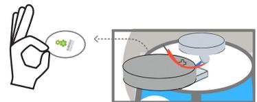
**D 3** To keep your robot turned off, put the sticker on the battery while making sure the red wire is not underneath the sticker.
